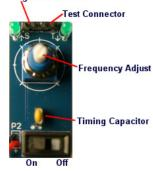
For use as just a signal source, connect the croc lead to the pin header marked 'S'. You can then connect the signal to whatever you wish (not exceeding specified limits) using the croc clips. Use the black clip for the common ground and the red clip as the signal source. The frequency of the output is adjusted by
