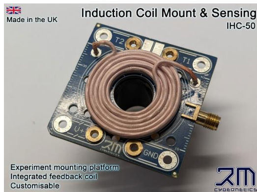
Figure 1: Example of mounted pancake coil
