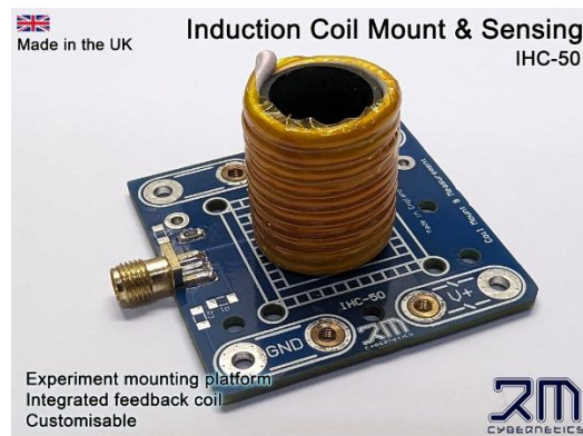
Figure 2: Example of mounted solenoid coil
