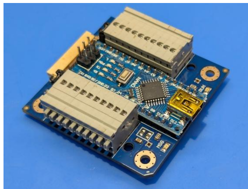
Figure 2: Example of mounted Arduino Nano clone
