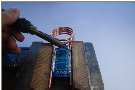
Figure 7: Soldering the PCB Edges
